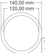
Footprint of the rings: 40cm2  $40 \text{ cm}^2 \times 3.5 \text{kg/cm}^2 = 140 \text{kg}$
