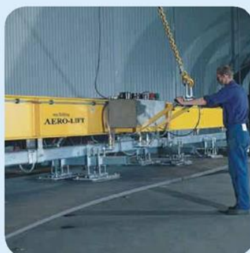
Fig. 1 Vacuum lifting unit, lifting capacity 32,000 kg
