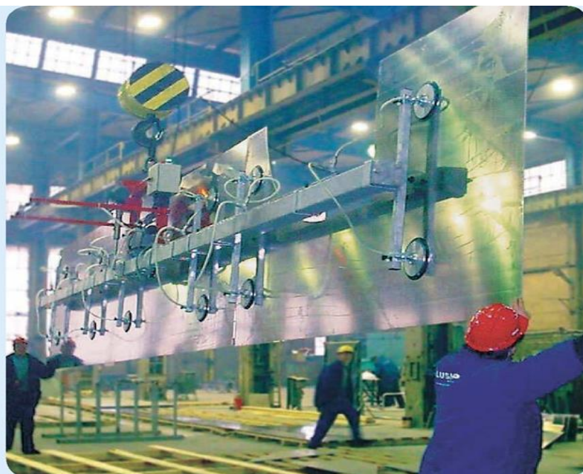
Fig. 1 90° pivoting coil lifter with multi-chamber suction plate
