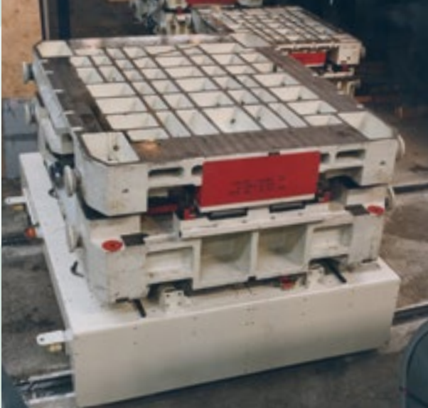
1 x 18 ton die change car on rails.
