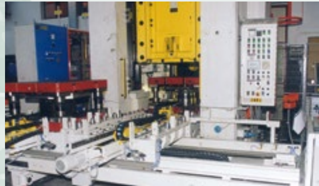
Example of a fully automated die change system with rail guided cars for 2 x 5 ton dies. In the press die lifters and the EAS MOD series clamp.
