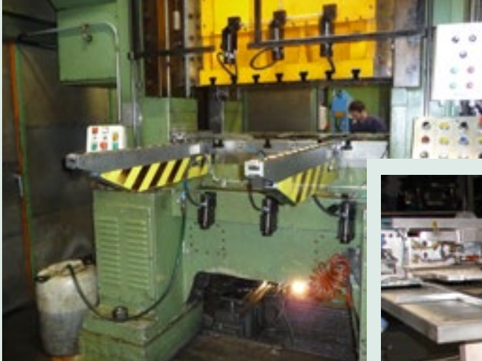
Complete retrofitted press with pre rollers, die lifters, ECA cylinders and parking stations.
