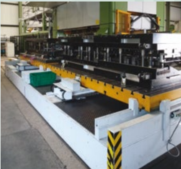
1 x 18 ton die change car on rails.
