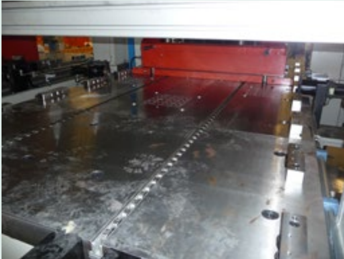
Magnetic clamping system in combination with air operated die lifters with rollers and guidings on the side.
