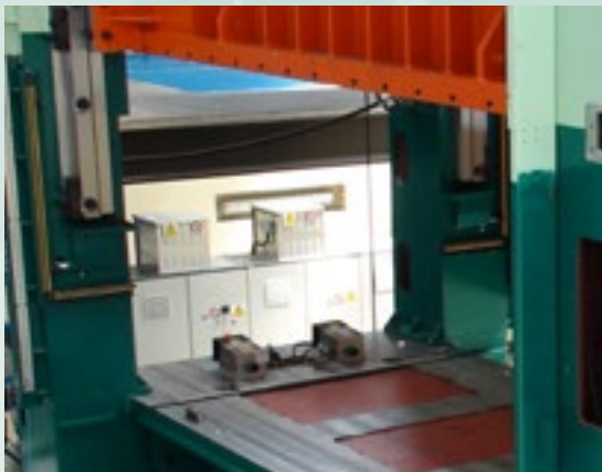
Wedge clamps for pressedbed clamping
