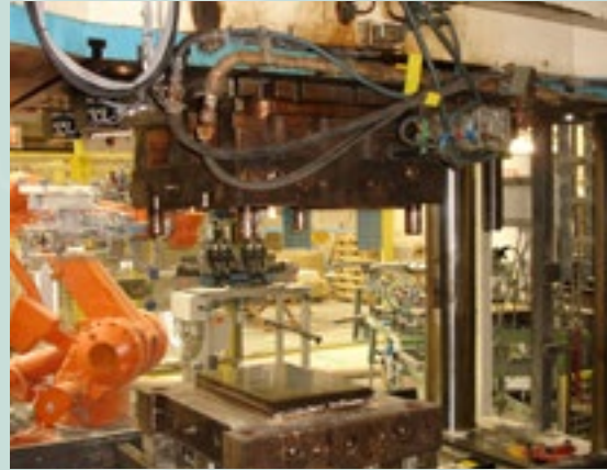
Hydraulic clamping, die lifting, pump unit with controls and pre roller solution
