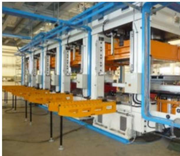
Group of presses equipped with Pressmag SP100 as well as guiding, air operated die lifters and pre rollers from one source, EASchangesystems.
