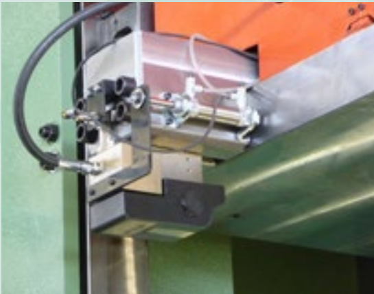
Rocker clamp with automatic movement by air cylinder
