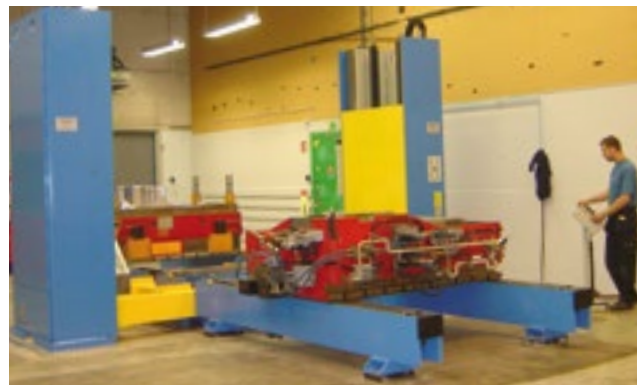
The upper half is lowered and moved outside for easy access and maintenance.
