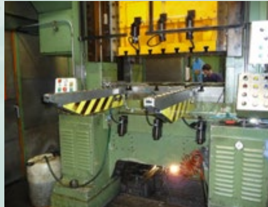
Large press with MHC clamps, multi couplers, die lifters and pre rollers
