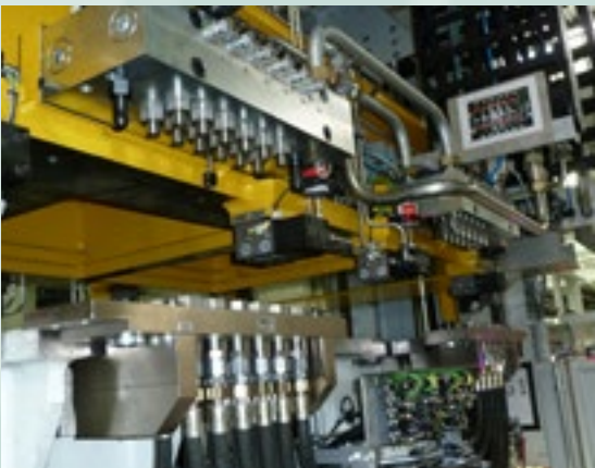
Hydraulic clamping, die handling, pump unit and controls as well as automatic multi coupler solutions
