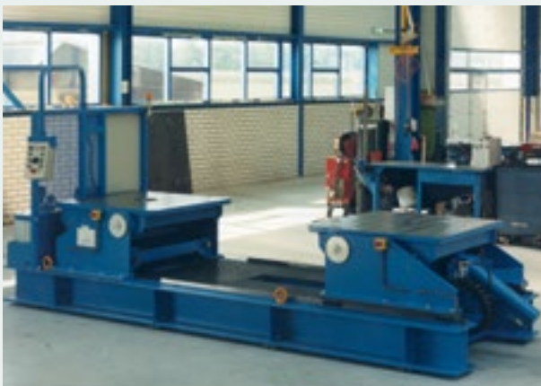
A small unit for dies up to 3 ton with both mounting plates turning.
