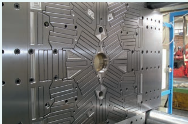
Pressmag HP on a 32000 kN (3200 t) machine
