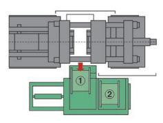
The complete mold changeover operation on this 1300-ton injection molding machine takes less than 50 seconds.
