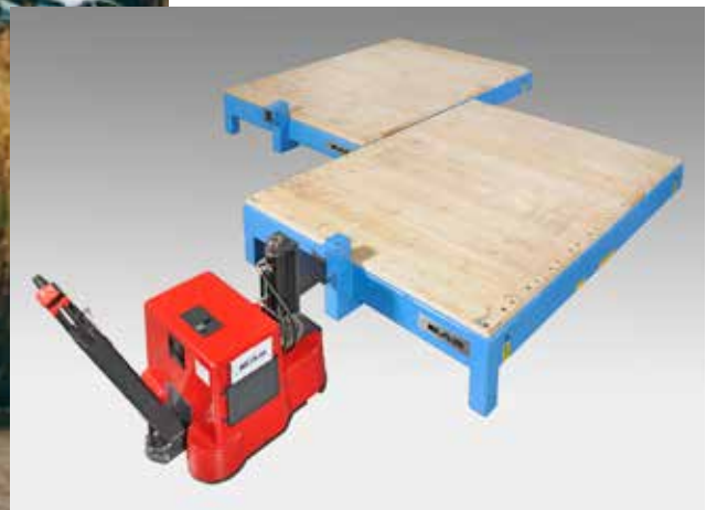
Tug unit to transport 20 t molds.
