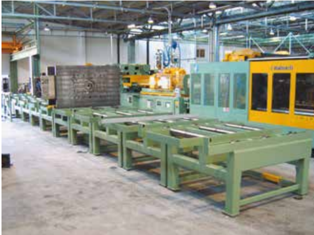
Mold storage racks in combination with a mold change car on rails. One of the storage racks is equipped with multi couplers and is serving as a pre heating station.
