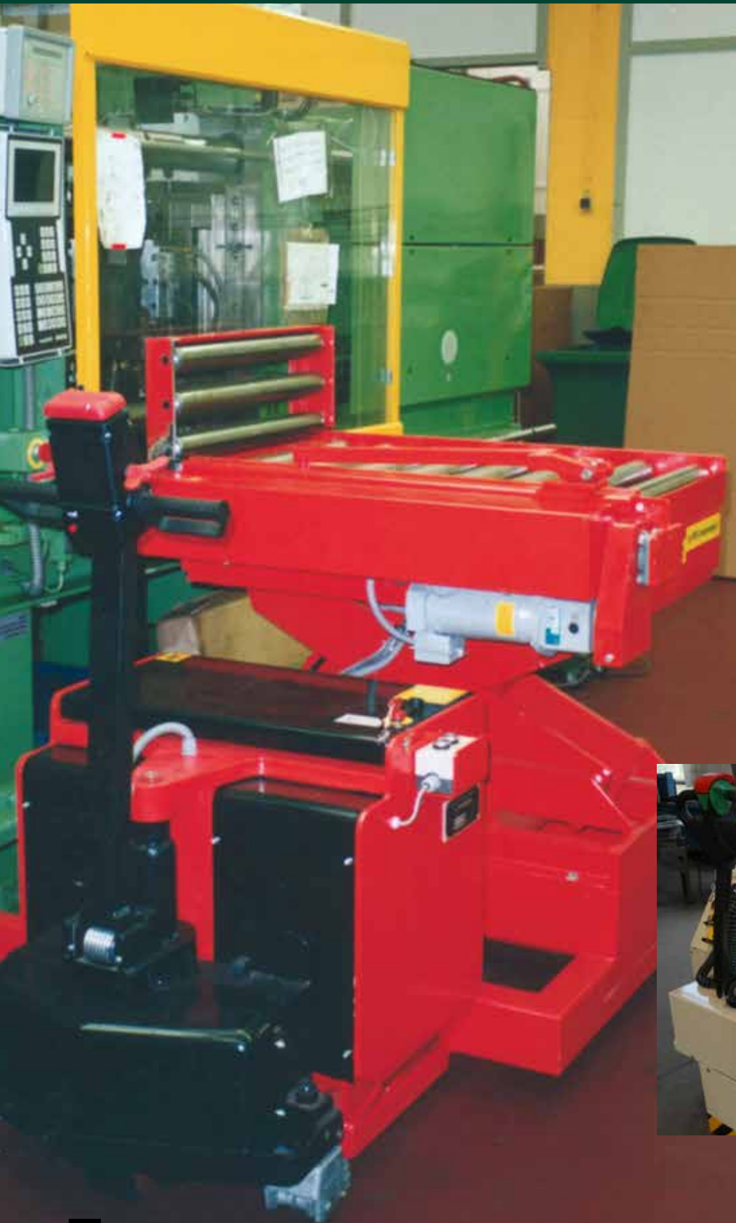
Mold change car with height adjustment 1 x 4 ton.
