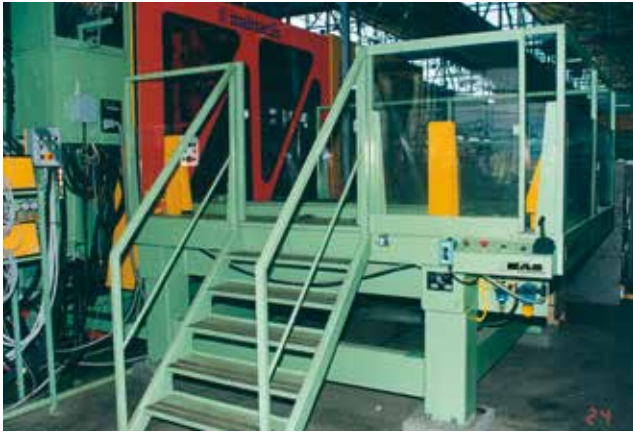
On an Italttech 1000 t injection molding machine EAS delivered the horizontal hydraulic adaptive clamping systems and a mold change table for molds of maximum weight of 40 t. Guides on the table allow the crane driver to easily position the large mold in a simple way on the table. An air driven push-pull spindle device moves the mold in and out the machine. All water, hydraulic and electric connections are made with manual multi coupler systems.
