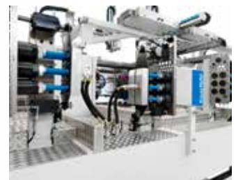
On this 900 t machine this table for 2 x 10 t molds enables the operator to change molds within 2 minutes.
