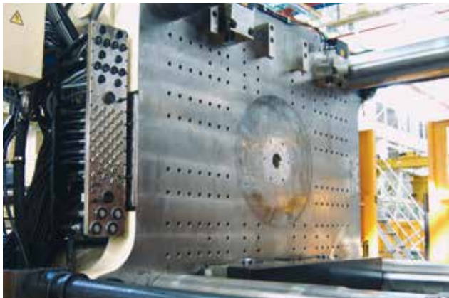
This multi coupler system for horizontal loading connects water and electric connections trouble free in less than 20 seconds. Another advantage of these multi couplers is that misconnections are being made any longer, which reduces the amount of bad products.
