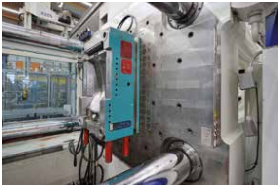
Pressmag SP on a 4000 kN (400 t) machine
