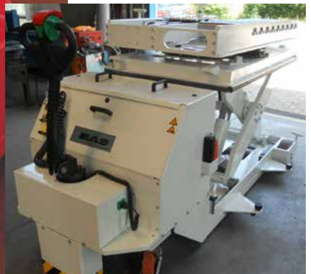
Mold change car with height adjustment 1 x 4 ton.
