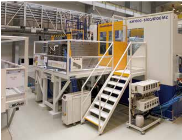
A 1000 t injection molding machine is equipped with an adaptive horizontal hydraulic clamping system, an ejector coupler, automatic multi couplers and a mold change table for one mold of maximum weight of 15 t.
