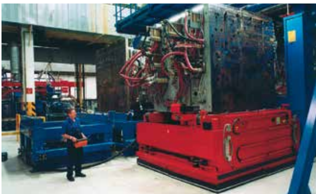
For extreme heavy molds as at this container manufacturer EAS installed this air floating system in combination with storage systems, a 3400 t and a 6000 t injection molding machine as well as an EAS inspection unit. The car can handle up to 150 t molds and the change over time is less than 30 minutes.
