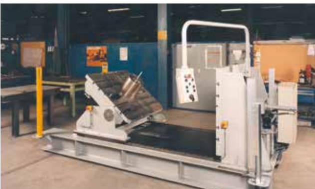
A small unit for molds of 2 t and with tilting platen. The control panel can be move around the unit by the operator. Safety mirrors as well as safety mat are also installed on this unit.
