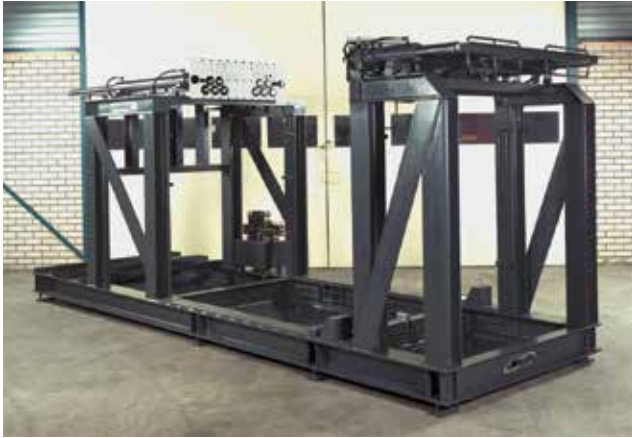
This separate mold pre-heating station is used to preheat 20 to 40 t molds outside the press.
