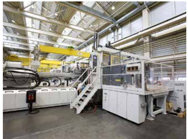
A table for 1 x 15 t mold with on one side the rollers with mold guidings, while on the other rollers molds with different dimensions can be placed. This table has a fixed operation panel. This table also features two guides to enable the crane operator to position the mold easily.
