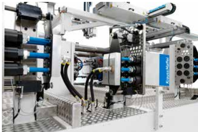
Integrated pre-heating station on a mold change table with automatic multi couplers equipped with leak proof hot oil couplers and electric connections.
