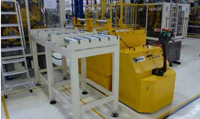
1 x 7 t with height adjustment but with powered transfer of the molds over the rollers.
