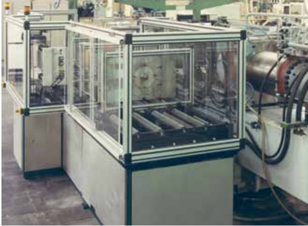
A fully automatic production cell with pre-heating station working with a 250 t injection molding machine.
