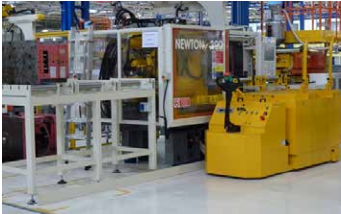
Electric driven 2 x 2 ton mold change car serving several machines and storage systems.
