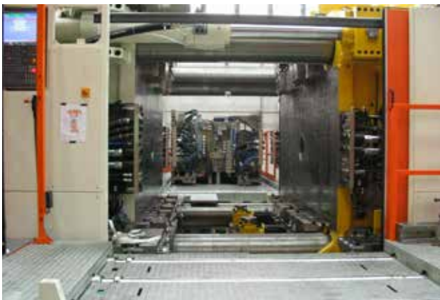
On both side of the machine a mold change table with pre heating and cooling down multi couplers.
