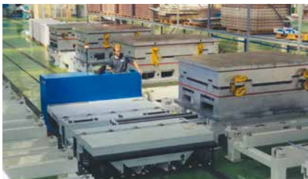
This electric driven mold change car for a large vertical press can bring the molds far away from the press to a special mold storage area. The molds can be stored left and right of the electric driven car. The driver has a camera and a monitor for exact positioning the car into the press. Changing and store molds between 10 and 20 t is in this way simple, fast and safe.
