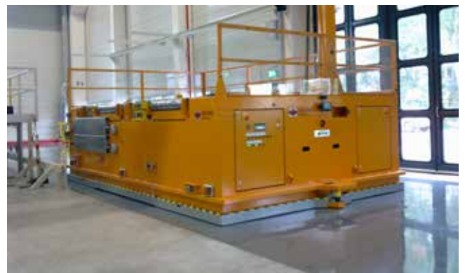
Air floating solutions can be very attractive for smaller mold handling requirements. It can also be combined with an electric drive system to travel longer distance. The operator can walk behind or even sit on board. Contact EAS for very creative solutions to your mold handling problems.
