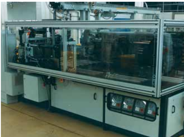
A 150 t machine with a 2 way 3 position mold change table, pre-heating, multi couplers, hydraulic adaptive clamping and an ejector coupler. The pre-heating equipment is stored under the table and can be easily reached.
