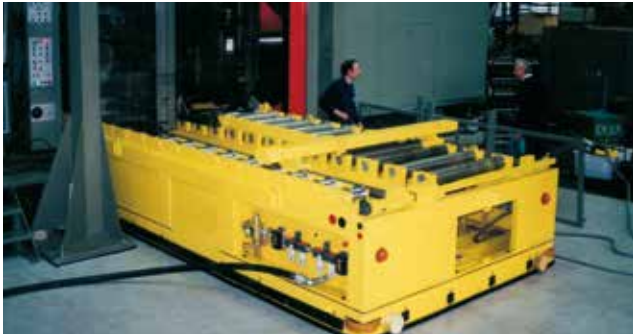
A 110 t mold is transported from its storage system to the injection molding machine or inspection unit. This customer, a producer of large plastic container, had no overhead crane available for such heavy weights and this solution enables them to change these molds within 35 minutes. The push pull mechanism is a simple spindle device, which pushes or pulls the molds in or out the large twin machine.
