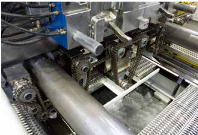
Inside the machine driven rollers on the fixed side.
