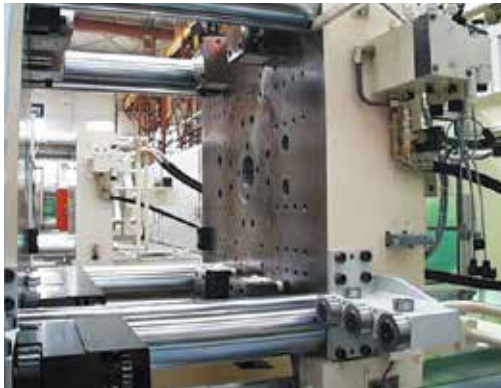
Powered roller system on a 500 t machine
