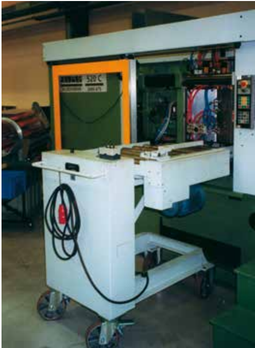
Our manual mold change car for one mold of max. 800 kg.
