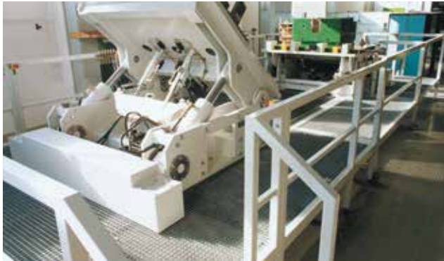
A German supplier of washing machines uses this inspection unit with two tilting platens for 20 t molds. The loading and unloading of the molds is done by an electric driven and air floating mold change car. The unit can also simulate core pulling movements and ejector couplers movements.
