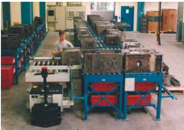
These horizontal mold storage systems are loaded and unloaded by means of electric driven mold change cars, on which either manual or automatically molds are placed. Underneath the molds is room for other mold related equipment.
