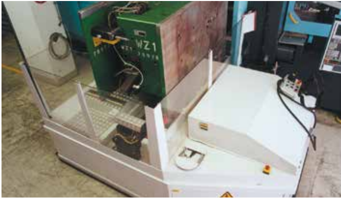
1 x 20 t with a combination of electric drive and air cushion floating for exact positioning in front of the machine, storage and inspection unit.
