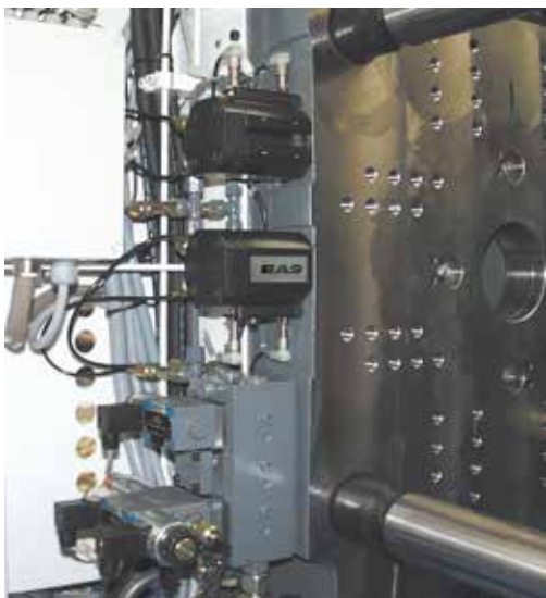
Hydraulic integrated clamping systems with 2 proximity switches for clamp position feedback.
