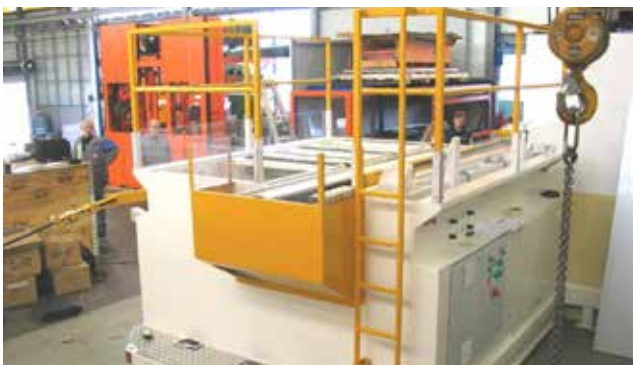
Space is very limited around the machines at this automotive supplier, two air floating cars for 1 x 20 t molds are used to change molds in less than 15 minutes.
