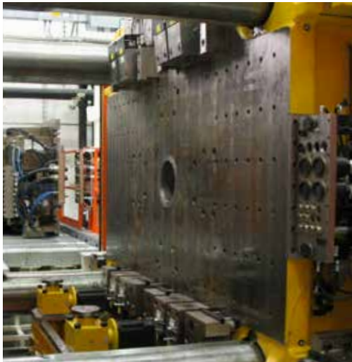
Horizontal loading of a 40 t mold from a change table into a 3200 t machine. The system included pre-rollers, centering cylinders, MOD 4010 clamps and multicouplers
